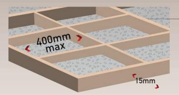
Construct the framework for your Gronodec to be installed on, using 6" x 2" joists around the perimeter and 4" x 2" joists in the centre. We recommend a maximum of 400mm between joist centres. Reduce this span to 350mm for areas of higher traffic or extra loading. Leave a 15mm gap between the edge of the framework and your walls. This allows air flow movement and heat expansion.
